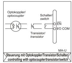
The output switch and EN have a reference to I/O COM. If the EN control signal is referred to PGND, a high-ohmic connection (e.g.  $10k\Omega$ ) must be made between I/O COM and PGND (This influences the galvanic isolation between PGND and I/O COM!).
