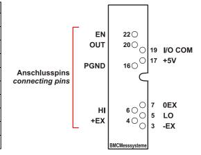
The pin assignment of the MA-UI corresponds to the 5B modules of Analog Devices and Burr Brown. An additional 0EX pin (pin 7) has been introduced as reference for +EX and -EX. If using a non-bmcm backplane that does not provide a relating connection, this pin has to be removed. Then, however, a reference of the ±EX pins is only possible via the LO pin with J7 being closed. This is a specific assignment of BMC Messsysteme GmbH. The 0EX pin is not connected in modules of other manufacturers.
