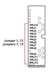
To prevent the modules from being damaged, close only jumpers required for the relevant application (see table chapter 2 and interfacing examples chapter 3). This applies especially to the power supply (close either J10 or J9 or J1!).
