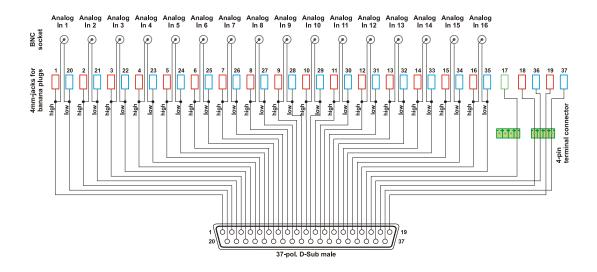
Always use only one connector type per channel, as double connecting may damage the board.
