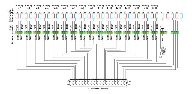
Always use only one connector type per channel, as double connecting may damage the board.
