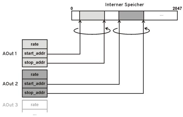
The module provides a memory for 2048 measuring values, in which any signal forms can be load. Each output channel of the MDA16-4i/-8i modules has its own controller, which can output any part of the internal memory. The part of the memory as well as the output frequency can be set for each channel separately.
